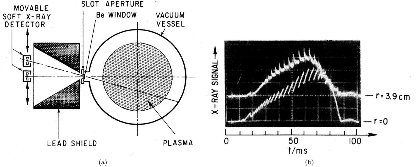
**Figure 1:** Experimental arrangement of x-ray detectors. The x-ray traces exhibit internal disruptions. Image is taken from (14).
